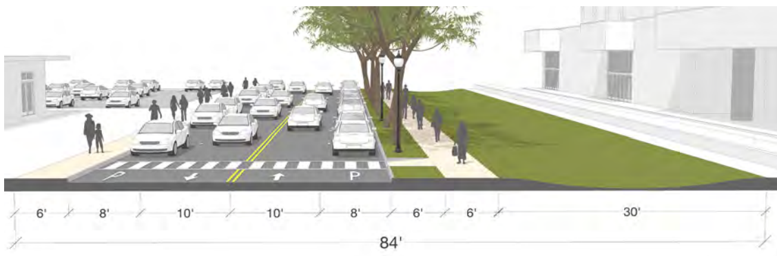
Figure 5.22 - 8th Ave Street Improvements - Reconstruction Option for Stormwater From Main to Missouri
