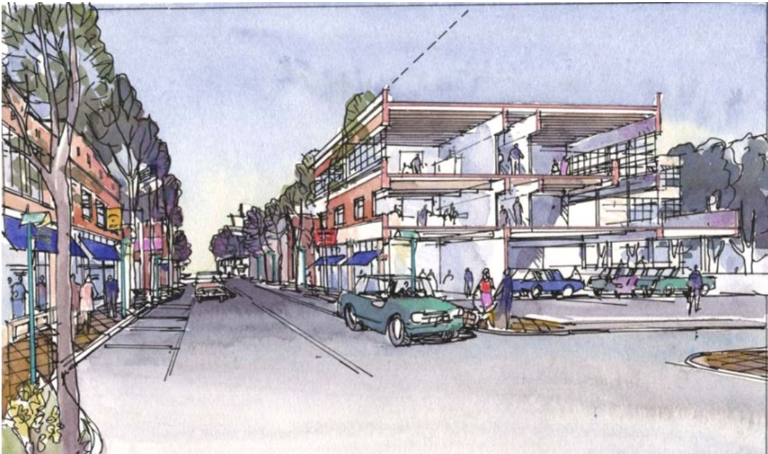
Attractive redevelopment that provides off-street parking would benefit downtown. This cross-section diagram shows mixed-use developments with parking located in an off-street court with alley access.
